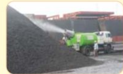
Mist Cannon used for Dust suppression in Stack-yard.
